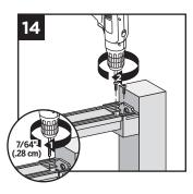
NOTE: Pre-drilling is recommended (7/64" [0.28 cm] drill bit) for attachment of railing to bracket.
