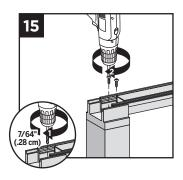
NOTE: Pre-drilling is recommended (7/64" [0.28 cm] drill bit) for attachment of railing to post.
