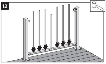
12. Place remaining balusters into holes in lower rail by snapping fully into place. In some cases, a **rubber mallet** may facilitate the fastening using **GENTLE** tapping.
