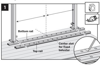
1. Position bottom and top rails between posts and align with bottom bracket. Align the center baluster slot in both rails with the middle of the span between posts.\* This will allow an equal number of baluster holes on each side of center slot. Mark bottom rail and top rail at each end (ensure both rails are centered between posts).
