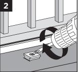
NOTE: Pre-drilling is recommended (1/8" [0.32 cm] drill bit) for attachment of base.
