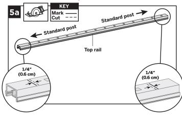
5a. Cut top rail to the measurement between the top swivel brackets. For standard-post-to-standard-post configurations this would be same dimensions as that of the bottom rail.
