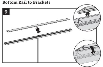
9. Attach "flat" bottom rail cover to bottom rail by first centering cover on bottom rail (this will allow gap on each end of bottom rail for placement into brackets). Align cover on one side of bottom rail in slot on side of rail. Then starting from one end of rail snap cover onto opposing slot working down the length of rail. In some cases, a **rubber mallet** may facilitate the fastening using **GENTLE** tapping.
