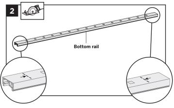
2. Cut bottom rail to the measurement between the bottom swivel brackets
