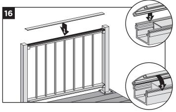
16. Attach "crowned" upper rail cover to upper rail by aligning cover on one side of rail. Then starting from one end of rail, snap cover onto opposing slot working down length of rail. A **rubber mallet** may facilitate the fastening using **GENTLE** tapping.
