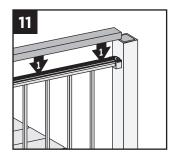
12. Secure 2" x 4" (51 mm x 102 mm) to top rail using Signature Cocktail Bracket (sold separately). Ensure that there is a bracket at each end of the railing section, then space brackets approximately every 24" and attach with 4 screws provided.
