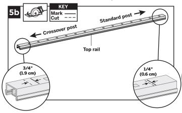
5b. Top rail must be cut differently on each side of the rail. Railing side that attaches to standard post should be cut 1/4" (0.6 cm) shorter than the mark to allow for fit into top rail bracket. Railing side that attaches to the crossover post should be cut 3/4" (1.9 cm) LONGER than the mark to allow for fit into the crossover post bracket.
