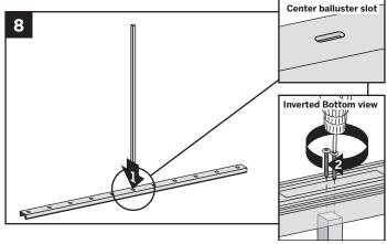
8. Attach shorter, center baluster in center slot in bottom rail using two #8 x 1-1/4" (3.2 cm) screws (provided).
