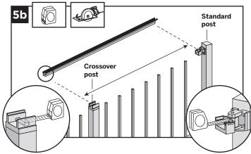
5b. When going from standard-post-to-crossover-post, measurement must be taken from inside of top horizontal swivel bracket to inside lip of crossover bracket (which is attached to top of crossover post).
