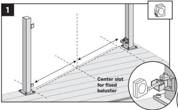
1. With brackets in correct swivel location, measure distance from inside of bracket to inside of bracket. ENSURE THAT BEFORE CUTTING, BALUSTERS HOLES ON BOTH BOTTOM AND TOP RAIL LINE UP. ALSO MAKE SURE CENTER BALUSTER SLOT IS AS CLOSE TO THE MIDDLE OF THE SPAN AS POSSIBLE. In some cases due to odd railing spans, the center baluster may need to be offset in one or the other direction to ensure there is enough room at both post locations for balusters to be placed.
