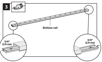
3. Slide rail insert out and cut 3/4" (1.9 cm) **FROM EACH SIDE** of insert, then slide back inside rail and center.
